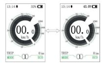
(7) "TRIP Reset" --- set reset function for single-trip distance
