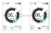
Switch mode between ECO and SPORT Press and hold (>2S) to switch riding mode into "ECO" or "SPORT".
